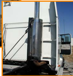
Step 3 (optional): Retrofit PM-control (Reduces replacement truck's PM by ~85%, w/ option for 25% NOx reduction)
