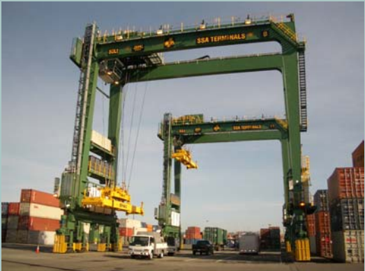
ZPMC Capacitor RTG Seattle, Washington 10% - 13% fuel reduction Significant emissions reduction
